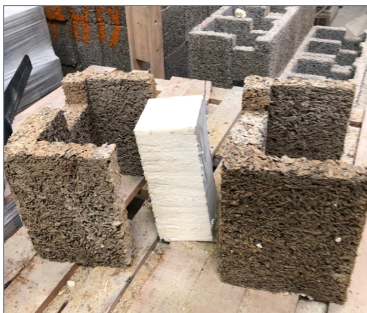
Intact offcuts of Durisol units and insulation that can be used elsewhere
