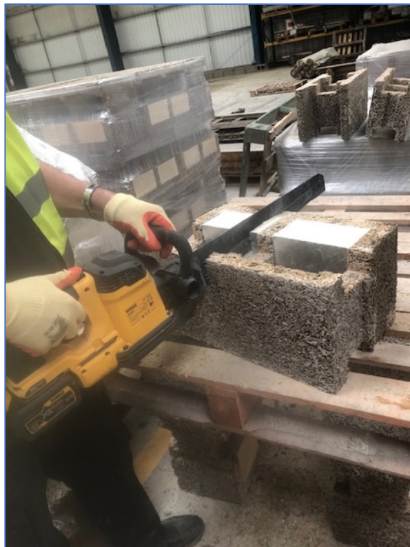
A unit being cut with an alligator saw
