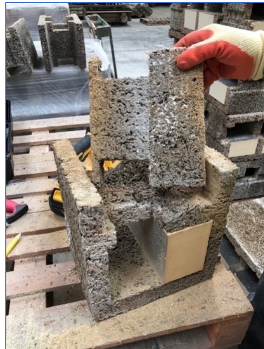
The additional web in a D300 Face Unit being removed
