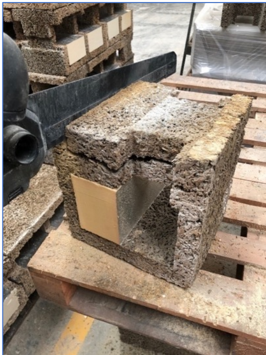
The additional web in a D300 Face Unit being removed
